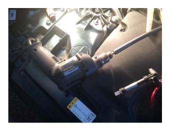
13. Snake drill extension down to place drill in supply line fitting on valve. Ensure that you do not turn drill on while you are trying to center the drill in the open. This is important: you need to make certain that the drill drops down into a hole before you start. Otherwise you might damage the seal.
