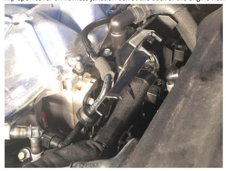
5. Gently lift harness from box and move about an inch to the front of the car to provide a bit more working space.
