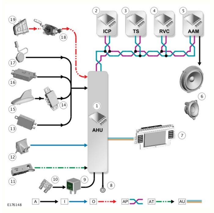
A = Hardwired; I = Composite Voltage Baseband Signal (CVBS); O = Local Interconnect Network (LIN); AP = Medium Speed (MS) Controller Area Network (CAN) comfort systems bus; AT = Universal Serial Bus (USB); AU = APIX2
