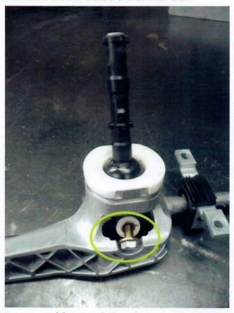
16.Remove old OEM shifter from inside the car.
