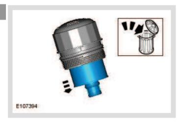
Remove and discard the oil filter element.
