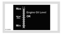
This display is now the live reading of the engine oil level.
