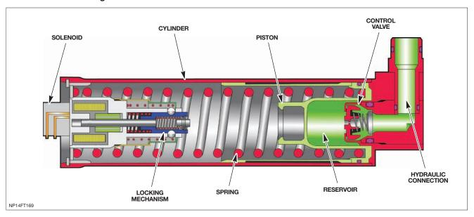
From the moment that the HIS is operated and the fluid is released, the shifting elements are subjected to hydraulic line pressure; this is then built further and maintained by the operation of the ATF pump once the engine is running.
