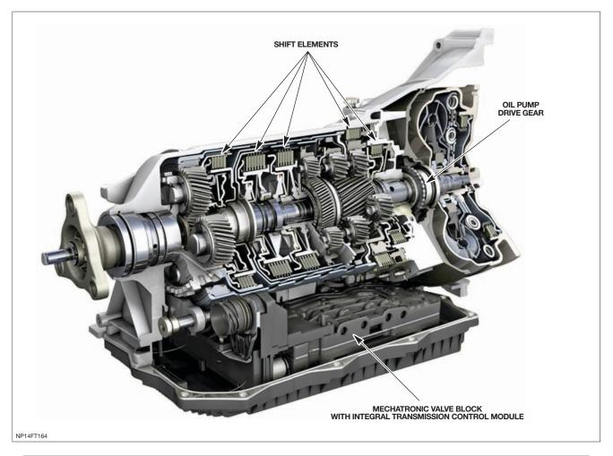
NOTE: The ZF 8HP transmission uses Shell L12108 transmission fluid (Jaguar part # JDE26444); the fluid specified for use with 6-speed transmissions is NOT compatible with the 8-speed unit.
