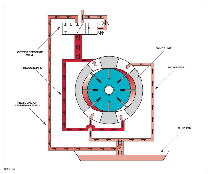
The ATF pump comprises a sprocket, a rear cover with bearing, a front cover with bearing, a cylinder, a rotor shaft, and a rotor with vanes. A pressure relief valve is fitted in the pressure outlet gallery from the pump but is not an integral part of the pump itself.
