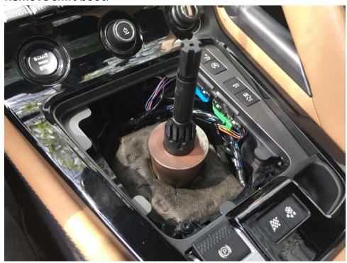
Remove counterweight (you may need to twist it in either direction to loosen, gently heating the counterweight might help as well):
