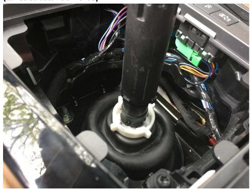
Remove both black rubber sleeves by lifting straight up:
