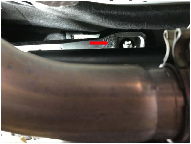
After removing the bolt, pull straight up on the OEM shifter from inside the car..
