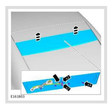
Release the retaining clips and disconnect the three electrical connectors.
