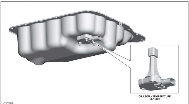
The continuous-mode sensor measures engine oil level and temperature. The oil level and oil temperature readings are taken and turned into a pulse-width modulated output signal.
