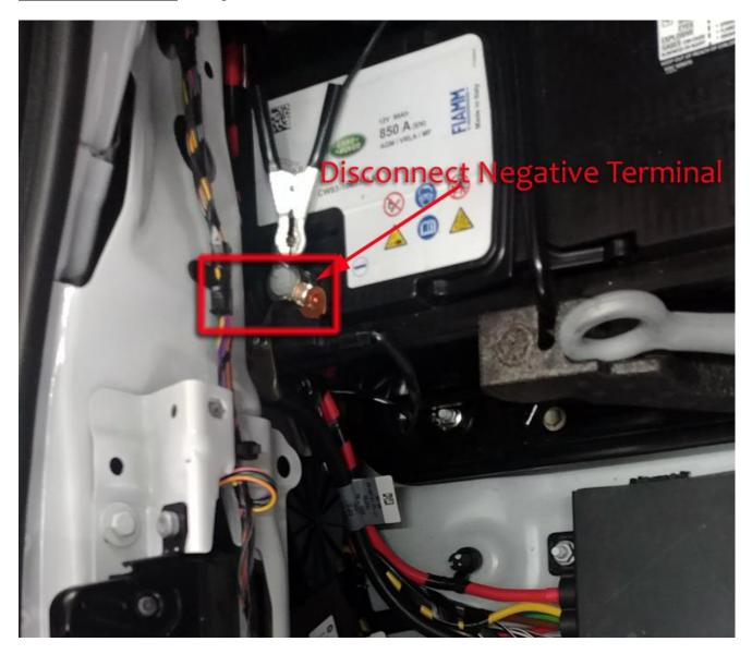
3. Add Terminal Disconnect Switch – You can get to it easily now that the panels are out. You remove the ground cable from the bolt/nut in the floor. Then you attach the ground cable to one end of this Disconnect Switch, then the other end goes on the bolt/nut in the floor pan as illustrated:
