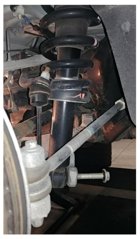
Do the reverse of all above steps to re-install everything. Make sure all fasteners are replaced and torqued. Jaguar recommends replacing all fasteners once removed. That is your call. After all is tight, replace wheel and lower car. Also note that most springs will "settle in" after a drive. So take it for a drive and give the car a day or so to settle to final ride height.
