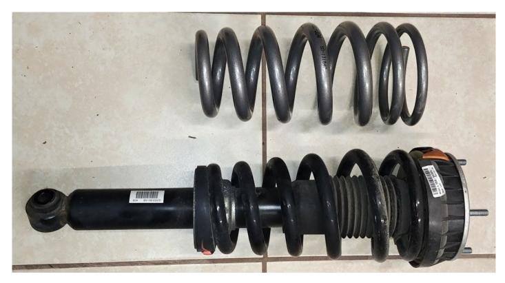
6. Replace Coil Spring – This will vary based on the tool(s) you use....But basically, you use a spring compressor, undo the top spring nut as you compress the spring. Release spring compressor. Remove old spring. Place new spring on strut. Compress spring. Re-install op retaining nut. Release compressor. Not there is a washer and rubber bumper inside of the tower cap. Be sure all parts are in place when re-installing. Put strut in Compressor, and compress to remoce retaining nut:
