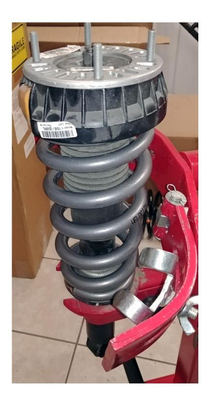
Re-Install in vehicle: Feed strut from bottom. Replace Link Rod bolt and Lower Strut Bolt. Replace Strut Tower nuts, and replace connector.
