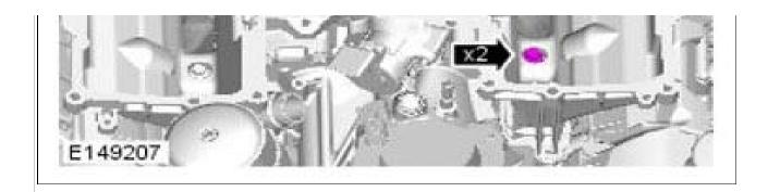
Special Tool(s): 303-1449-01, 303-1449-02 Torque Specification:**25 Nm**
