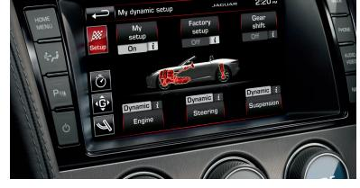
If your F-TYPE is fitted with Configurable Dynamics this can be set up to your own favoured dynamic driving settings using the configurable dynamics screen.
