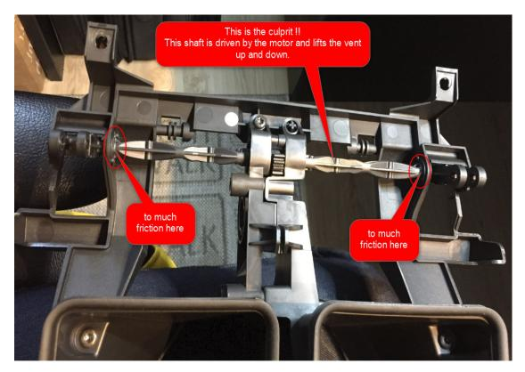
The plastic is expanded -> the bearing is to tight -> the shaft cannot turn smoothly.
