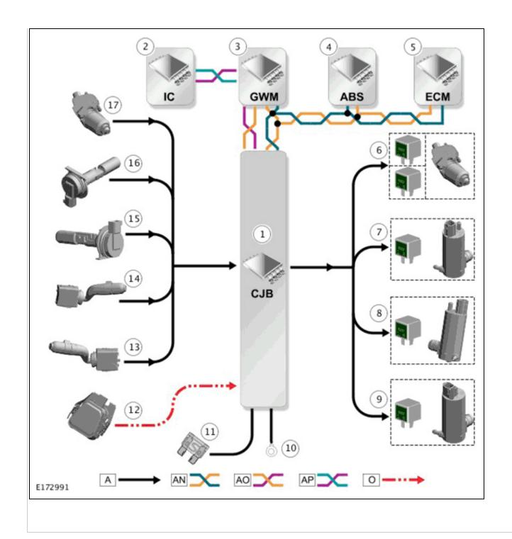
A = HARDWIRED; AN = HS (HIGH SPEED) CAN (CONTROLLER AREA NETWORK) POWERTRAIN SYSTEMS BUS; AO = MS (MEDIUM SPEED) CAN BODY SYSTEMS BUS; AP = MS CAN COMFORT SYSTEMS BUS; O = LIN (LOCAL INTERCONNECT NETWORK) BUS.
