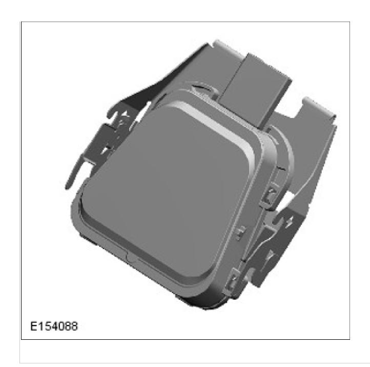
The rain/light sensor is located at the upper edge of the windshield, behind the rear view mirror. The sensor is mounted with a clip onto a bracket, which is bonded to the inner surface of the windshield during manufacture. If
