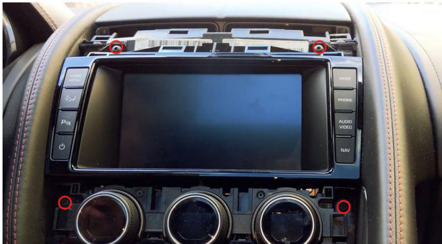
3. Remove those bolts those holding screen dash from each sides
