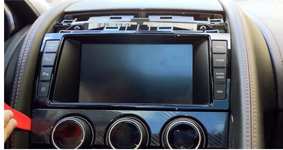
2. After removal of the cover, do the same with climate control cover
