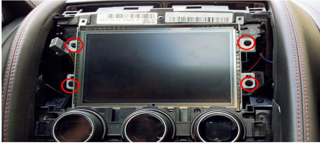
5. Remove those 4 bolts holding display
