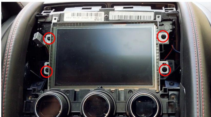
5. Remove those 4 bolts holding display
