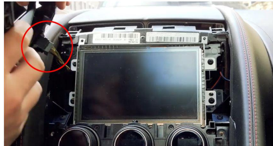
4. Remove the facia from the screen, after disconnecting the power cable for buttons
