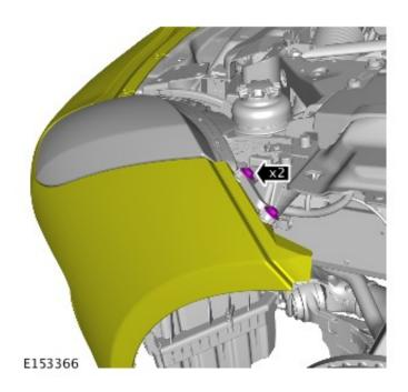
**40.** If the gap is too small and out of specification, pull the bumper forward from the bottom until the correct size gap is achieved and then tighten the bolts shown.
