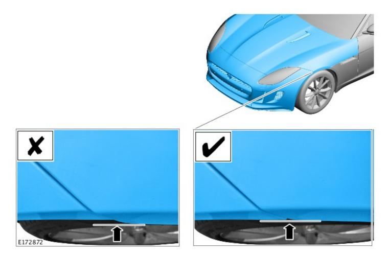
**7.** Check the area shown for correct bumper cover-to-hood alignment.
