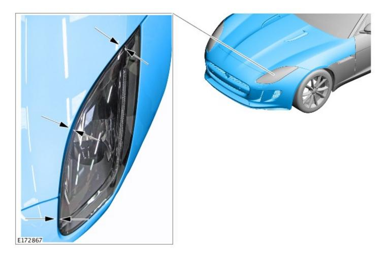
**5.** Check area shown for correct bumper cover-to-hood alignment - ' $\checkmark$ '.
