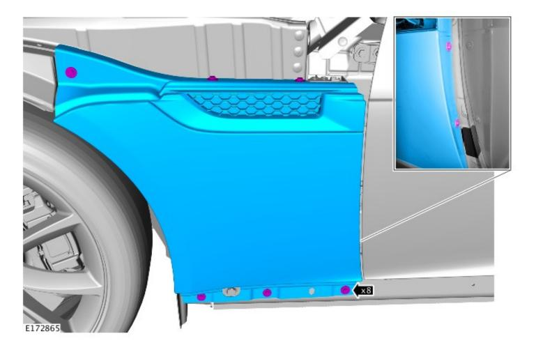
**12.** Locate the rocker panel moulding back onto the vehicle (do not install the fixings).
