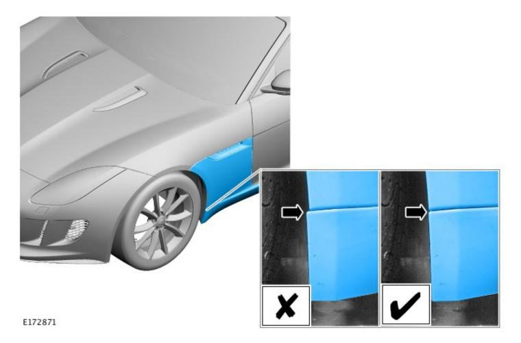
**3.** Check the area shown for correct front fender-to-hood alignment -  $\checkmark$ .
