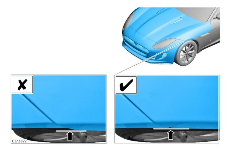
**44.** Install the fender splash shield; see TOPIx Workshop Manual, section 501-02: Front End Body Panels - Fender Splash Shield.
