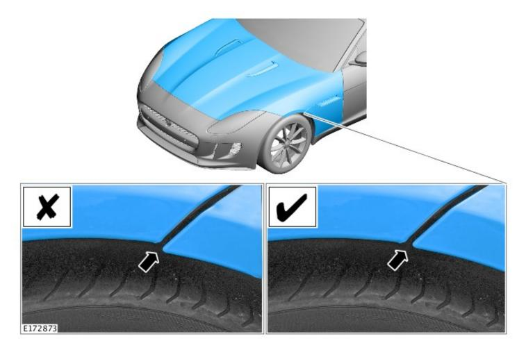
4. Check the area shown for correct headlamp-to-hood alignment.
