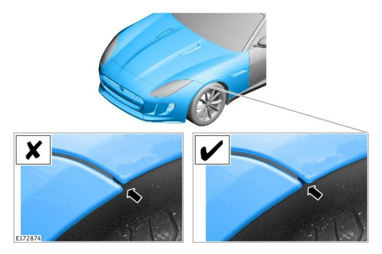
**6.** Check the area shown for correct bumper cover-to-hood alignment - ' $\checkmark$ '.
