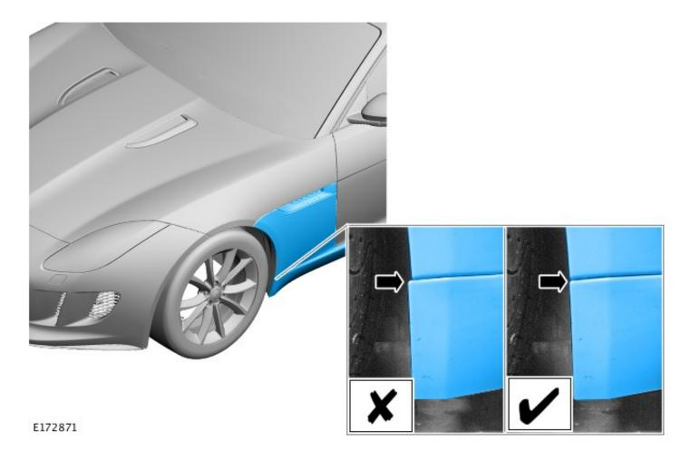
**14.** Align the fender with the front edge of door.
