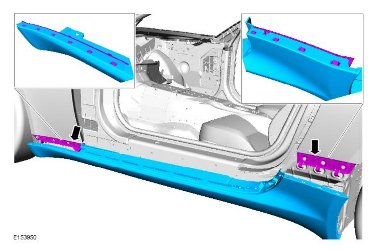
**13.** Align the fender with the front edge of the rocker cover to check the alignment of the fender - ' $\checkmark$ '.
