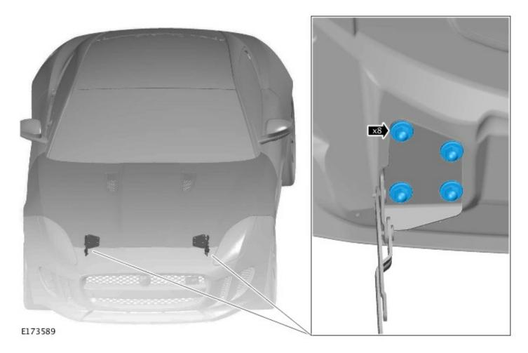
**22.** Align the hood with the doors; see TOPIx Workshop Manual, section 501-26:Vehicle Specific Information and Tolerance Checks > Description and Operation.
