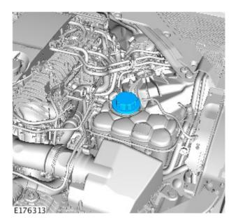
Remove the engine coolant expansion tank pressure cap.
