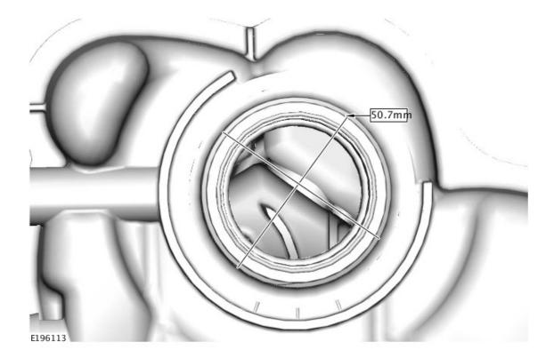
Check the dimensions of the engine coolant expansion tank threaded neck in the two positions shown.
