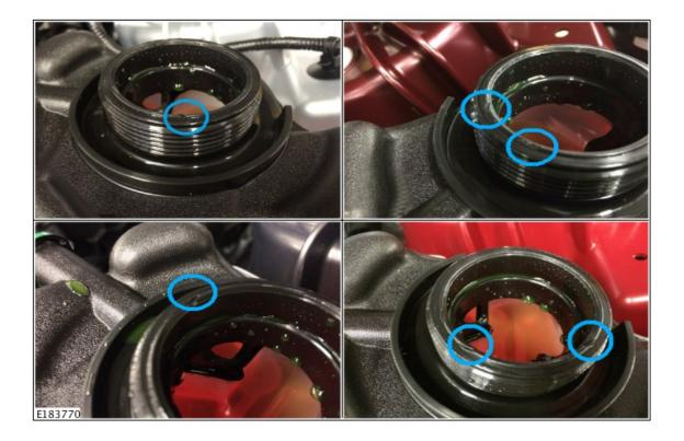
Visually inspect the sealing bead on the engine coolant expansion tank neck to check for damage.
