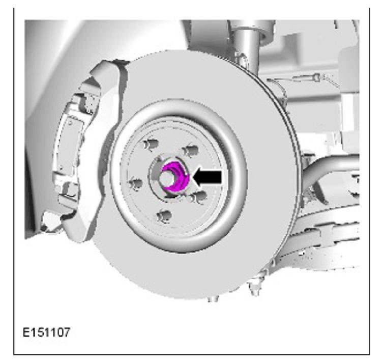
Torque Specification: 300 Nm
