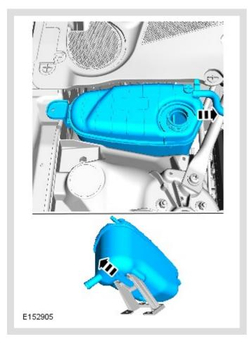
Raise the coolant expansion tank 50mm from its original position.
