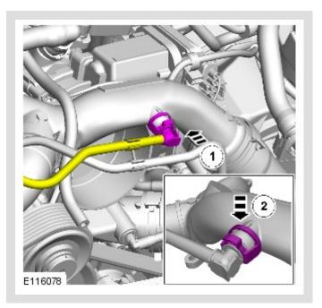
Once coolant is visible from the outlet, connect the pipe.
