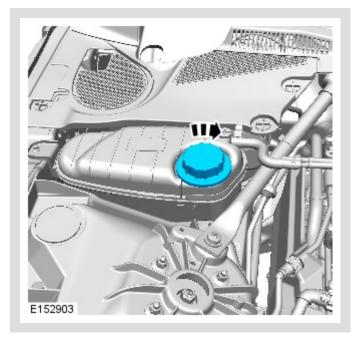
Install the coolant expansion tank cap while the engine is at idle.
