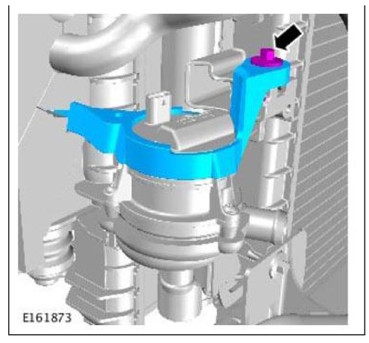
Torque Specification: 9 Nm
