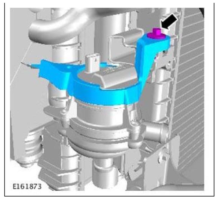
Torque Specification: 9 Nm
