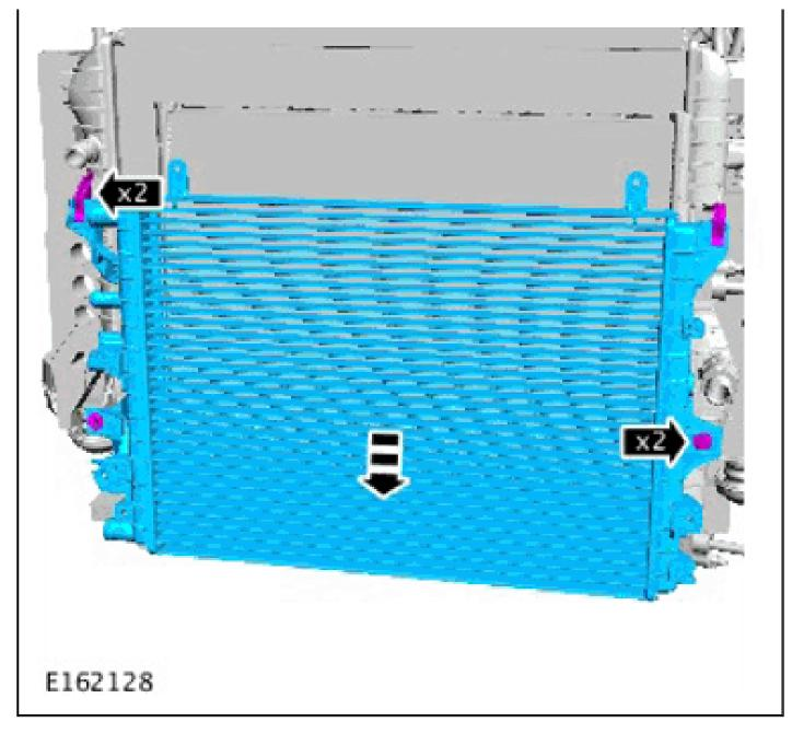
Torque Specification: 7 Nm
