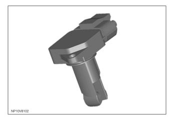
The measured air mass flow is used in determining the fuel quantity to be injected in order to maintain the sto-ichiometric air/fuel mixture required for correct operation of the engine and exhaust catalysts. Should the device fail, there is a software backup strategy that will be activated once a fault has been logged.
