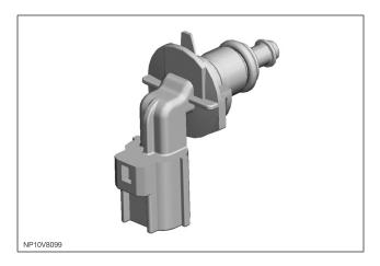
The ECT sensor is vital to the correct running of the engine, as a richer mixture is required at lower block temperatures for good quality starts and smooth running, leaning off as the temperature rises to maintain emissions and performance.
