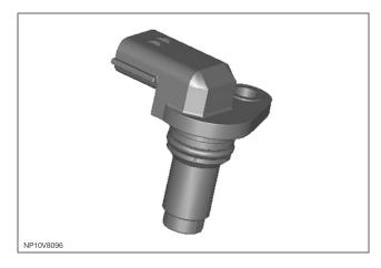
There are four common sensors, one per camshaft.
