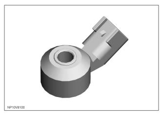
Each sensor monitors engine knock by converting the engine block noise into a suitable electrical signal, which is then transmitted back to the ECM via a twisted-pair cable. The signal is processed within the ECM to identify the data that characterizes knocking.
