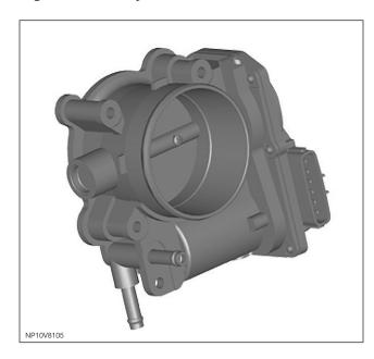
This value is input into the ECM and the throttle is opened to the correct angle by means of an electric direct current (DC) motor integrated into the throttle body. Movement of the motor is achieved by changing the PWM signal to the DC motor, allowing it to be operated in both directions.
