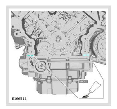
Apply RTV sealant (Loctite 5901G) to the areas shown.
