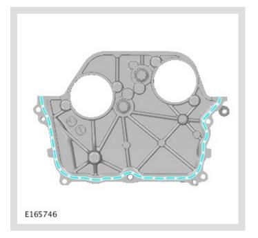
Apply RTV sealant (Loctite 5901G) to the areas shown, and tighten the bolts within 7 minutes.
