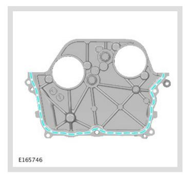
Apply RTV sealant (Loctite 5901G) to the areas shown, and tighten the bolts within 7 minutes.
