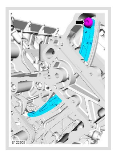
Remove the timing chain guide.
