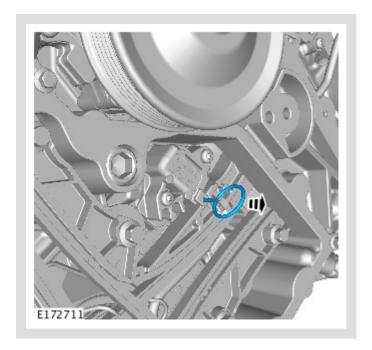
Remove the timing chain tensioner retaining pin and release the timing chain guide.
