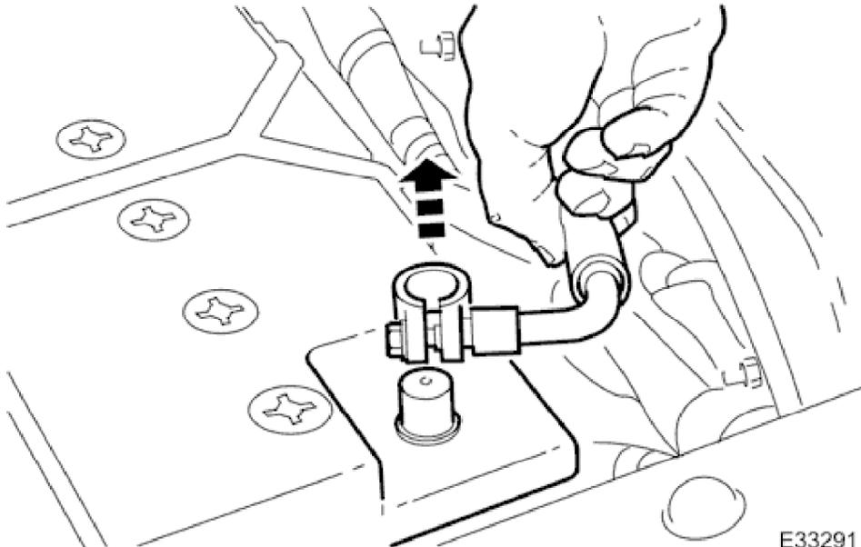
1. Disconnect the battery ground cable.
