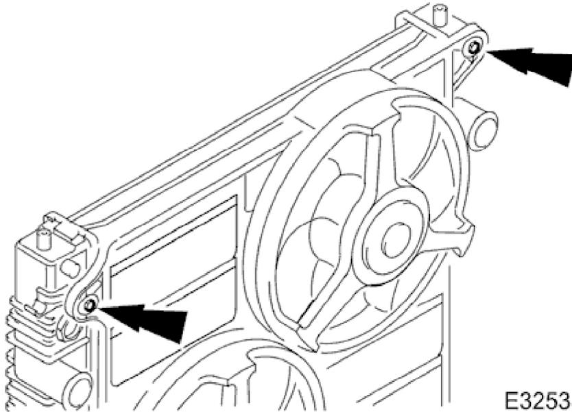
4. Remove the two bolts which secure the fan and motor assembly to the radiator.
