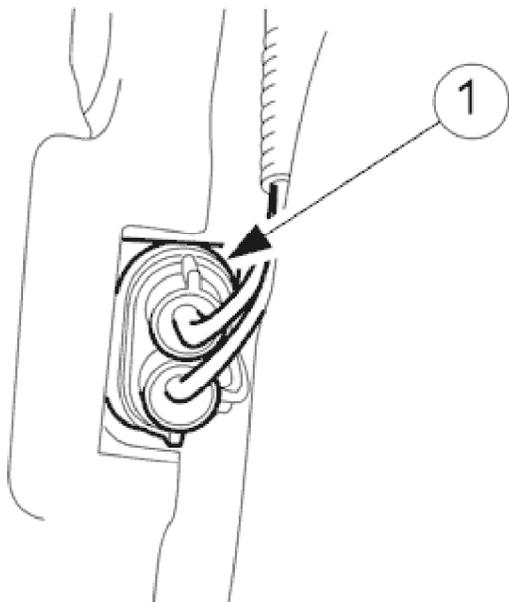
3. Disconnect the harness multiplug from each cooling fan.
