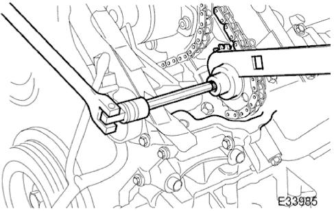
12. Remove the bolt which secures the sprocket to the exhaust camshaft.• Move the sprocket forward from the camshaft boss.
