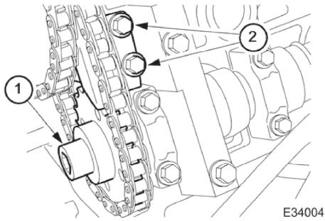
4. Install the chain tensioner to the engine.
