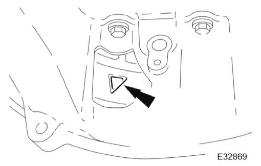
6. Rotate the crankshaft until the triangular arrow indent on the drive plate is visible through the access hole; confirm that the timing flat on each camshaft is uppermost.
