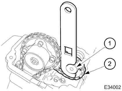
1. Install the sprocket to the secondary chain.
