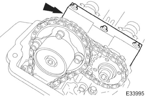
9. Install the camshaft locking tool 303-530 to Bank 2 camshafts, aligning the shafts slightly as necessary.
