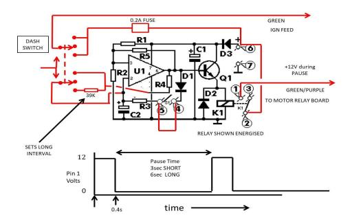
Delay Timer Schematic and Waveform
