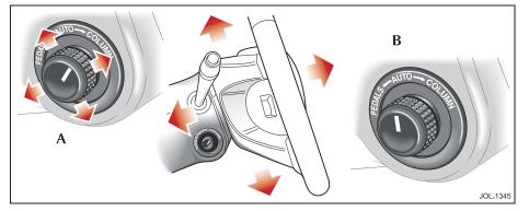
Exit – If the ignition key is in position '0' and the driver's door is opened or if the ignition key is removed, the steering column will move to the uppermost tilt position and the seat will move slightly rearwards.
