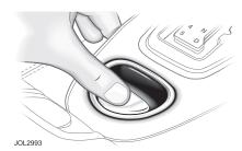
**To release parkbrake**: The ignition switch must be in position 'II', apply the footbrake and push the parkbrake switch down.
