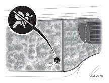
The front passenger seat is equipped with a sensor that determines the occupancy status by measuring the weight on the cushion and changes the passenger airbag deployment status.
