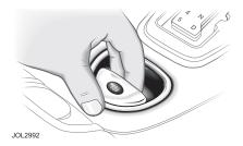
To apply parkbrake: Pull the parkbrake switch up and release. The warning light in the instrument cluster will illuminate.
