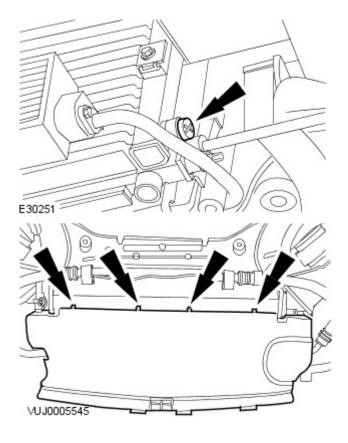
5. CAUTION: Do not over tighten the radiator drain plug. Failure to follow this instruction may cause damage to the vehicle.
