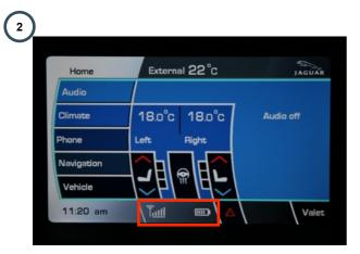
**Home** menu shown indicates phone connected (paired & docked). Signal strength and battery condition shown on lower edge of screen.
