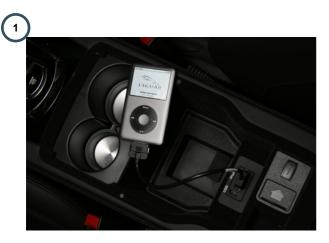
The Portable Audio Interface connections are located in the cubby box.
