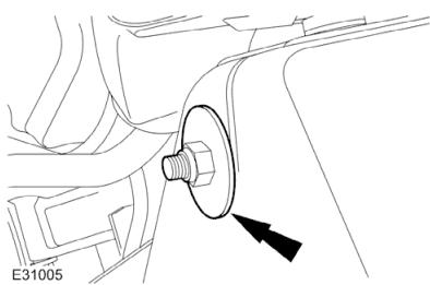
7. Remove the upper arm retaining nut.
