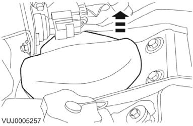
7. Remove the shock absorber and spring assembly mounting cover plate.
