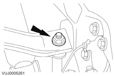
2. Remove the stabilizer bar link retaining nut.
