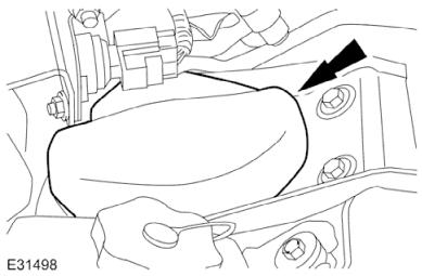
3. Install the shock absorber and spring assembly mounting cover plate.
