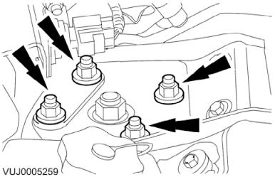
Install the shock absorber and spring assembly.
