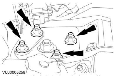
9. Remove the shock absorber and spring assembly.
