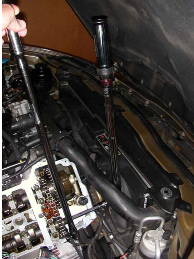
Fig. 7 Torque wrench, Timing Chain Tensioning Tool and breaker bar in place during removal of sprocket-to-camshaft bolt
