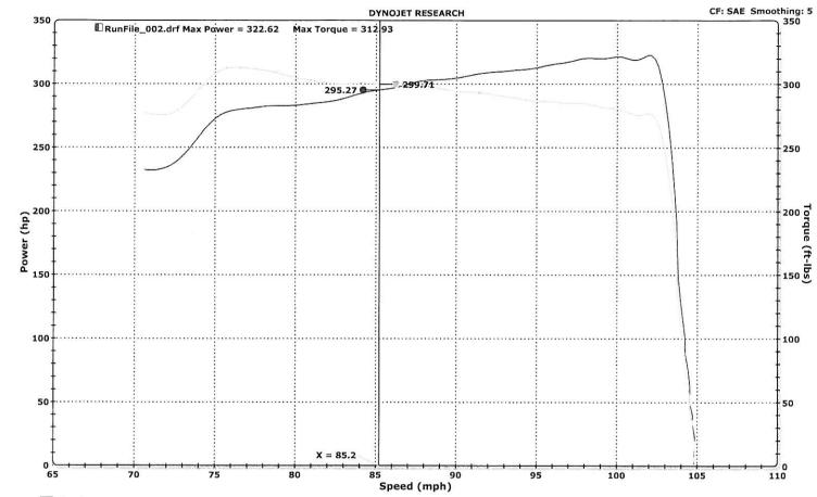
RunFile\_002.drf - 9/25/2009 10:27:58 AM Run Type: RO Run Conditions: 82.84 °F, 29.55 in-Hg, Humidity. 11%, SAE: 1.00 Max Power = 322.62 Max Torque = 312.93
