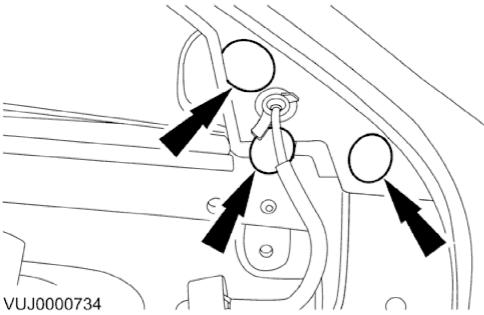
4. Remove the rear view mirror screw covers.
