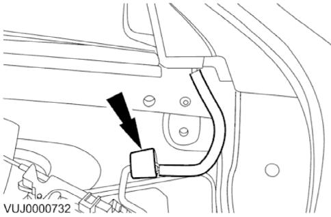
2. Disconnect the rear view mirror electrical connector.
