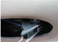
When the lower position tag is released a small part of the retaining tag location window on the chrome cover will fracture as the force to release it is applied - see photo below.
