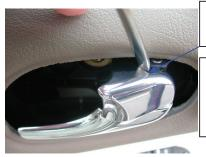
Apply force here first to release lower outer location tag
