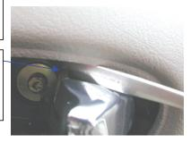
Applying force in the order and in the positions shown, releases the cover from the two small retaining tags on the flag lever which is part of the door release assembly.
