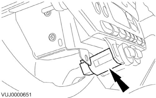
3. Disconnect the heated seat electrical connectors.
