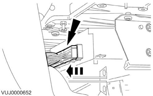
4. Disconnect the climate control unit electrical connectors.
