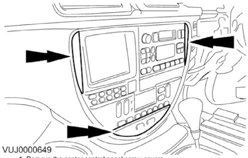
1. Remove the center control panel screw covers.
