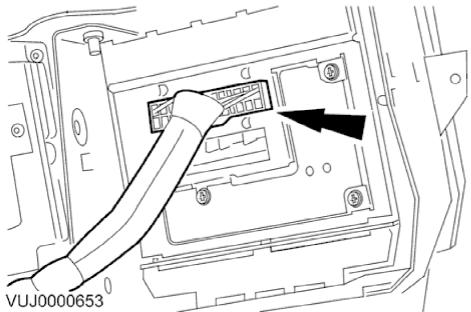
5. Disconnect the satellite navigation screen electrical connectors.
