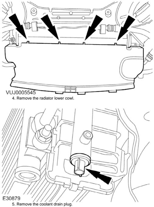
• Drain the coolant into a suitable container.
