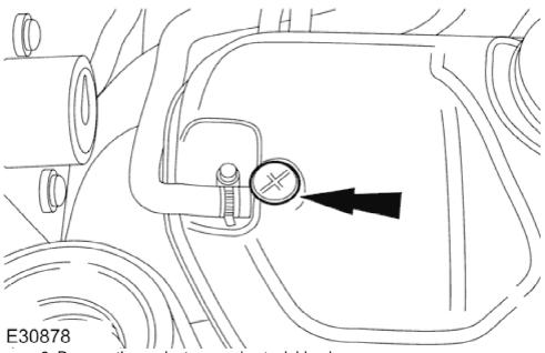
9. Remove the coolant expansion tank bleed screw.
