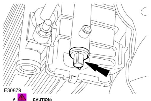
CAUTION: Do not over tighten the drain plug. Failure to follow this instruction may cause damage to the vehicle.
