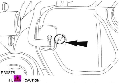
Do not over tighten the coolant expansion tank bleed screw. Failure to follow this instruction may cause damage to the vehicle
