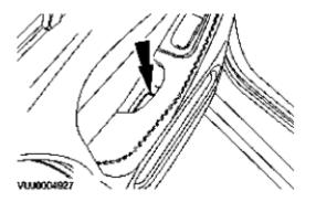
3. Remove the rear door trim panel retaining screws.
