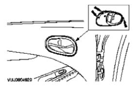
2. Remove the rear door trim panel retaining screw cover.
