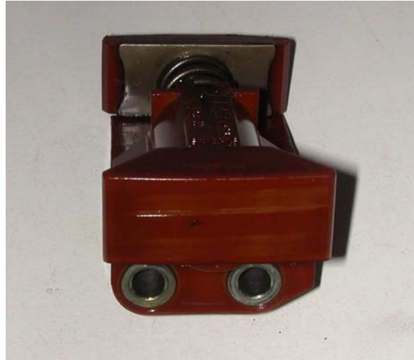
Fig. 10 Slipper surface showing minimal wear
