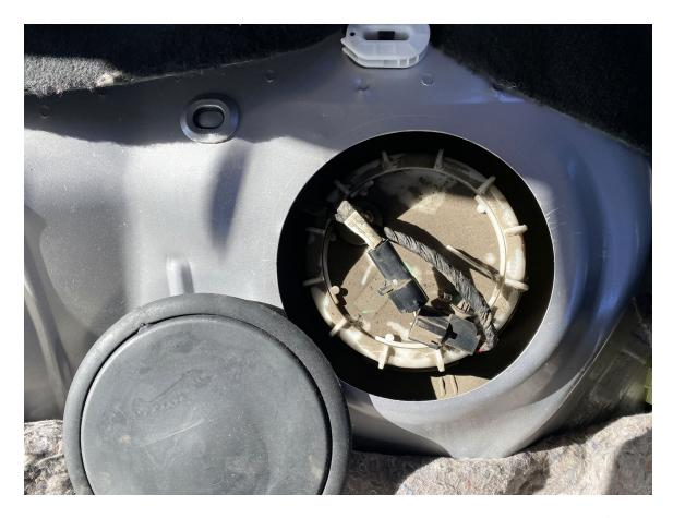
At this point I would recommend moving the carpet back over the seat latch to avoid any fuel splashes.
