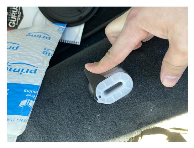
Once the Rear seat bottom is removed you will see a black circular cover on the right side. This can be a bit frustrating to remove but nothing that can't be done. You will want to gently pry the edge and lift up. Once removed it will reveal the sending unit. Go ahead and unplug the sending unit plug and move the connecters to the side.
