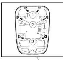
2. CAUTION: Make sure the overhead console retaining tangs are released in the order shown. Failure to follow this instruction may result in damage to the component.
