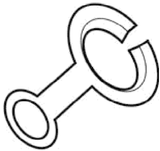
205-461 Halfshaft seal protector 205-461
