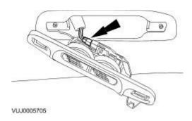
15. **NOTE:** Left-hand shown, right-hand similar. Detach the front passenger assist handle retaining screw covers.
