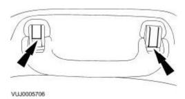
16. **NOTE:** Left-hand shown, right-hand similar. Remove the front passenger assist handle.
