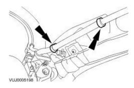
19. Remove the roof opening panel rear drain hose.
