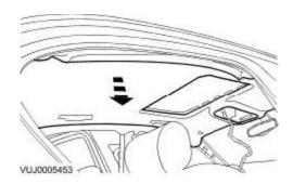
18. Detach the roof opening panel rear drain hose retaining clips.
