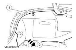
5. Detach the roof opening panel rear drain hose retaining clip.
