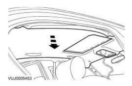
15. Detach the roof opening panel front drain hose.
