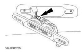
12. **NOTE:** Left-hand shown, right-hand similar. Detach the front passenger assist handle retaining screw covers.
