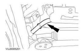
16. Remove the roof opening panel front drain hose.
