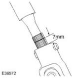
29 . Fully tighten the new lower column pinch bolt, install the new fastener and tighten to 35 Nm.
