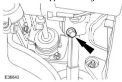
7. Detach the lower steering column universal joint from the steering gear.
