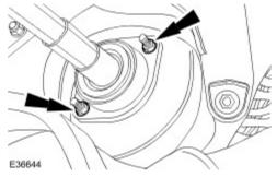
11. Remove the lower steering column.
