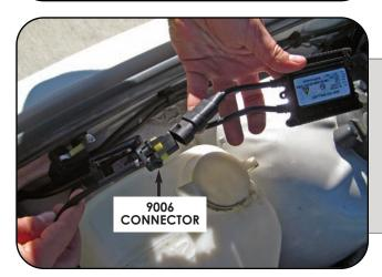
Then plug the 9006 connector on the adapter harness to the ballast. Finally mount the ballasts in a dry, flat, clean location. And plug your car headlight wiring connector back into the headlight.
