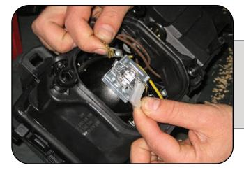
Disconnect the positive and negative female spade connectors from the headlight by pulling firmly away from the low beam bulb.
