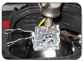
Using a Dremel tool, carefully grind the metal bulb retainer slightly. Go slowly and test fit the bulb as you go. Repeat grinding as many times as it takes for the H1 HID bulb to fit.
