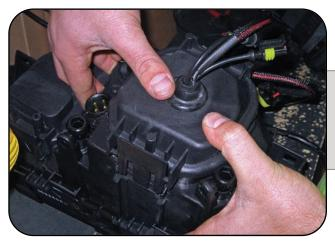
Once all the wires are connected, reinstall low beam dust cover onto headlight housing.
