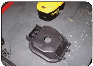
Pictured is the drilled low beam dust cover.
