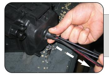
**GENTLY** pull on the wires while holding the rubber grommet firmly in place. This will eliminate any slack inside the headlight housing, giving you more wire to work with.
