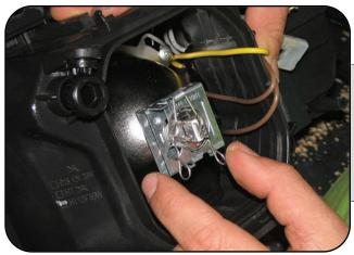
Next, pinch and release the metal retaining clips which will allows the OEM H1 low beam bulb to be removed.
