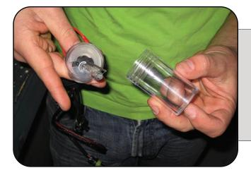
Remove the H1 HID bulb from the protective plastic casing and screw cap. Do not touch the bulb with your bare hands. If you do, be sure to clean the bulb with rubbing alcohol prior to installation.
