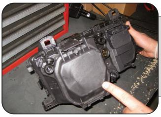
Once OEM headlights are removed from the vehicle, it will be much easier to do your HID install. Pictured is the low beam dust cover, this will require minimum modification in order install your H1 HIDs correctly.
