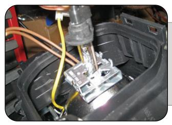
Carefully test fit the H1 HID bulb on your headlight housing. If the HID bulb does not slide in effortlessly, DO NOT FORCE IT. You will need to open up the metal bulb retainer slightly with a Dremel tool.
