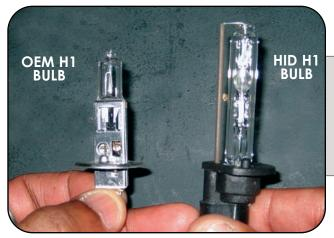
Pictured is the comparison between your OEM H1 vs. HID H1 bulb. Note the difference in size.
