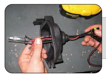
Carefully pass the H1 HID bulb and wiring through the modified low beam dust cover. The rubber grommet stays to outside of the dust cover.
