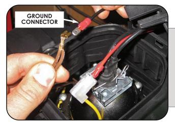
Plug the male spade adapter cable connector (the **RED** wire coming through the grommet) into your female spade connector from inside your headlight housing.
