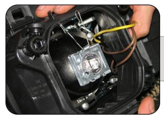
Pictured is the metal retaining clip fully unlocked.
