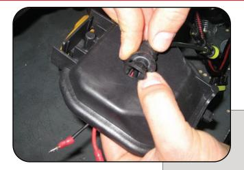
Pinch half of the rubber grommet through the 7/8" hole, sealing your low beam from the elements.
