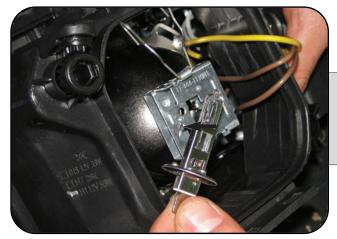
Gently remove the OEM H1 bulb out of the headlight housing.
