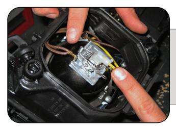
Once the low beam dust cover is removed, your low beam bulb and positive/negative connectors will be exposed.
