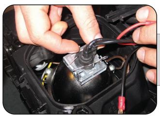
Secure the H1 HID bulb in the headlight housing by reinstalling the metal retaining clip.
