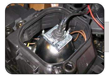
Pictured is the H1 HID bulb installed correctly in the headlight housing.
