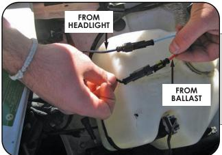
After reinstalling your headlight with new HID installed back on your car, plug the corresponding AMP connectors from the ballast to the HID bulb.
