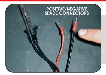
Coming through the rubber grommet on the H1 HID bulb side there will be a positive and negative spade connectors. These will be plugged into your female spade connectors inside your headlight.
