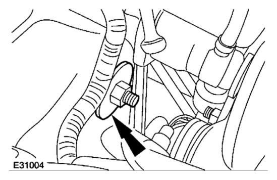
6. **CAUTION:** The final tightening of the Upper arm retaining nut must be carried out with the vehicle on its <u>wheels</u>.
