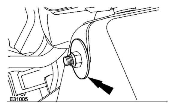
5. **CAUTION:** The final tightening of the Upper arm retaining nut must be carried out with the vehicle on its wheels.
