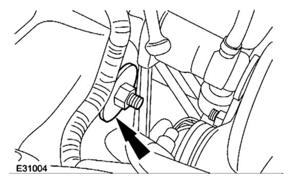
5. Remove the upper arm retaining nut.
