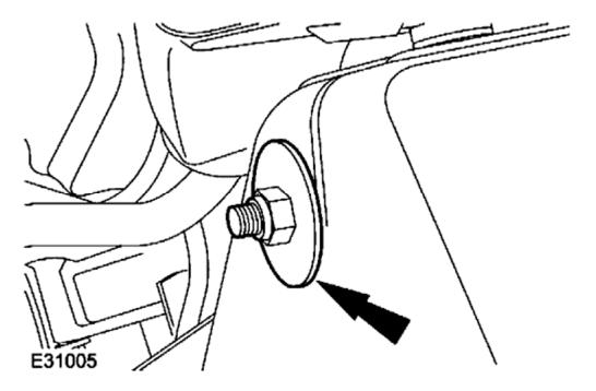
7. Remove the upper arm retaining nut.
