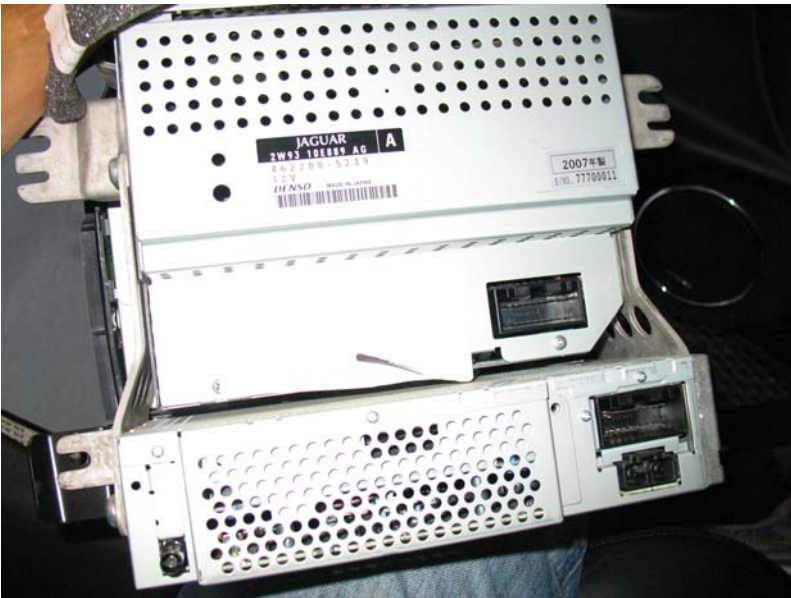
Rear view of head unit. Main connections are all different
