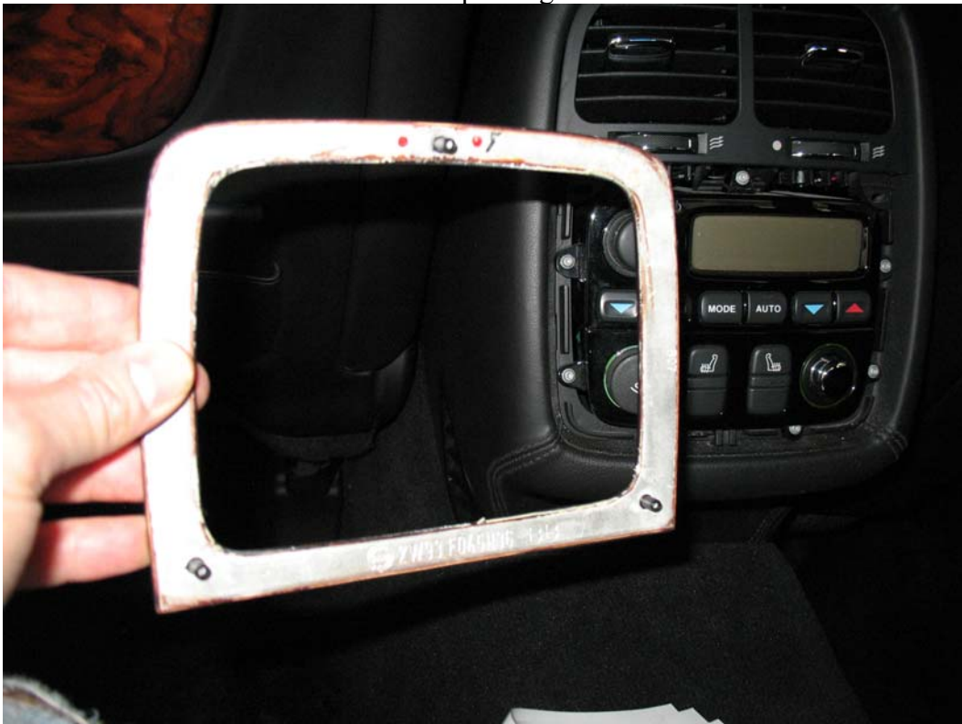
Likewise so is the trim around the rear passenger controls
